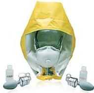
Grainger Qualitative Fit Test Apparatus,
